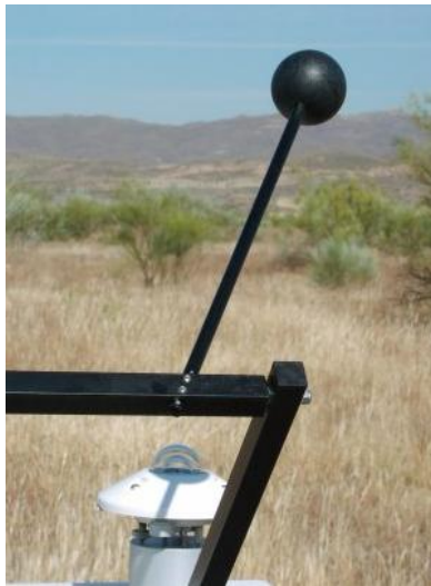
Figure 3.11: Pyranometer with shading ball device for diffuse measurements [19].
