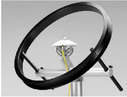
Figure 3.10: Pyranometer with shading ring device for diffuse measurements [18].
